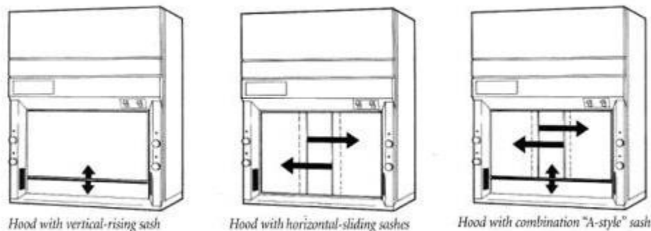
Figure 1: Illustration of the types of chemical fume hood sashes.
