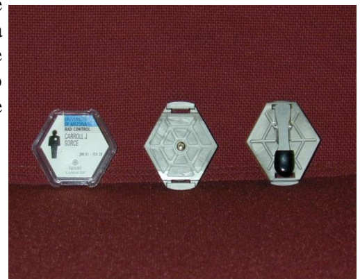
Figure 10: Badge Dosimeter (showing front of unit and front/back of holder)
