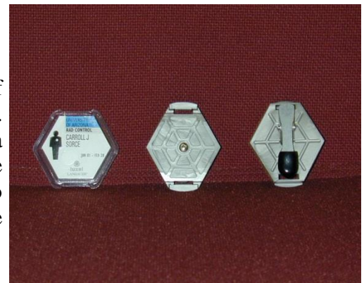
Figure 6: Badge Dosimeter (showing front of unit and front/back of holder)
